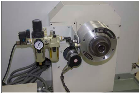
Figure 1-18: FRL Filter-Regulator-Lubricator installed in front of the anti-rotation plate.
