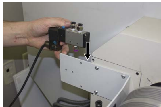
Figure 1-17: Solenoid behind the anti-rotation plate.
