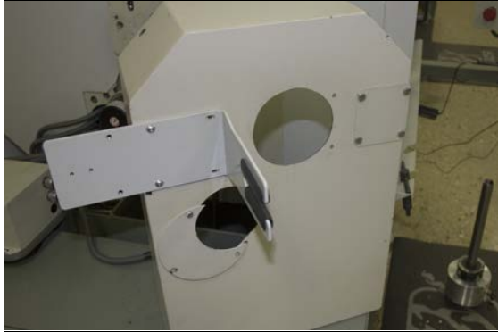
Figure 1-8: Example of an anti-rotation bracket installed on a belt guard cover.
