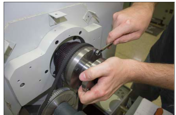
Figure 1-11: Adapter spacer installed on the spindle pulley.
