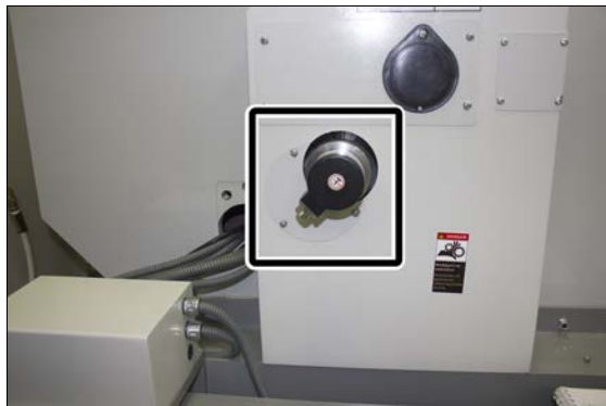
Figure 1-5: Rotary encoder on the belt guard cover.
