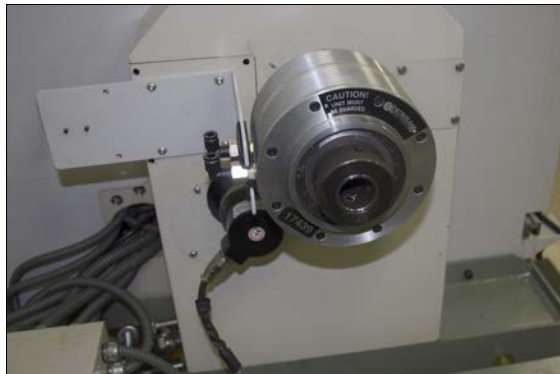
Figure 1-12: Pneumatic cylinder assembly put into the spindle.
