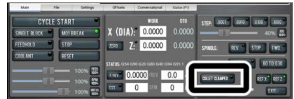
Figure 2-3: Example of the Collet Clamped button with the light off.
