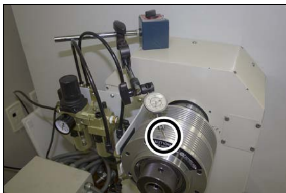
Figure 1-27: Example of a magnetic dial indicator put on a pneumatic cylinder.
