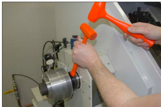
Figure 1-28: Example of using two dead-blow hammers to align an Automatic Collet Closer Kit.
