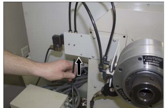
Figure 1-25: Example of an air connection at port P on the solenoid.
