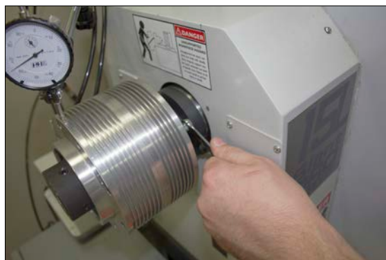
Figure 1-29: Tighten the mounting flange on the pneumatic cylinder.
