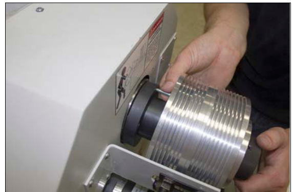
Figure 1-14: Pneumatic cylinder assembly installed on the adapter spacer.
