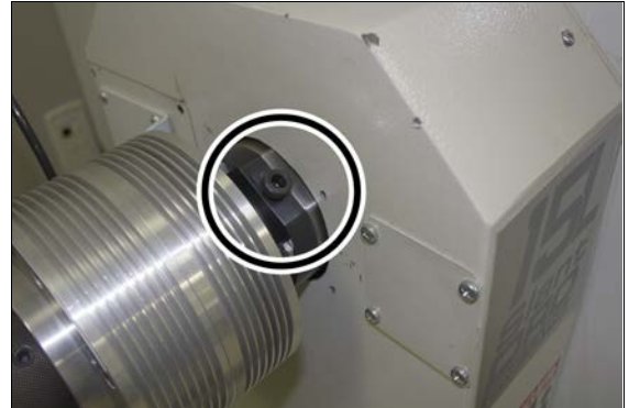
Figure 1-13: Example of an aligned thumb screw on a pneumatic cylinder assembly.
