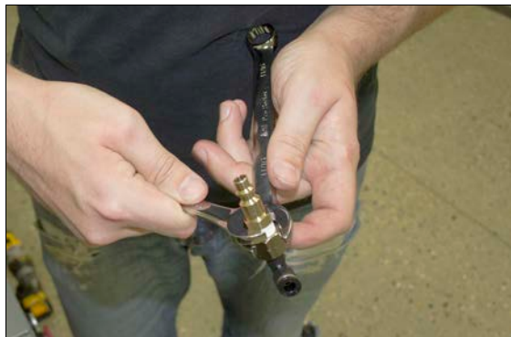
Figure 1-26: Quick-connect fitting installed in the elbow fitting.
