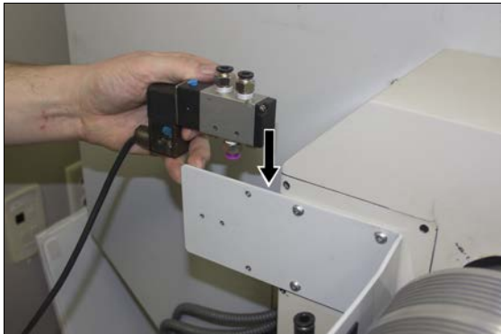
Figure 1-23: Solenoid behind the anti-rotation plate.
