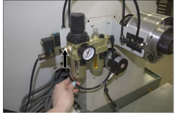
Figure 1-20: Example of an air connection at the output port on the FRL Filter-Regulator-Lubricator.
