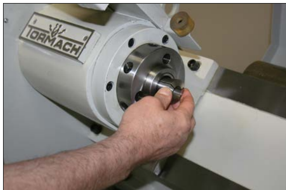
Figure 1-16: Collet installed into the 5C insert.
