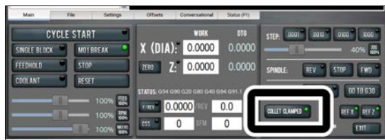
Figure 2-1: Example of the Collet Clamped button with the light on.
