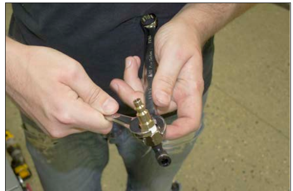
Figure 1-21: Quick-connect fitting installed in the elbow fitting.
