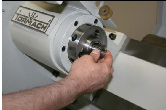
Figure 2-5: Collet installed into the 5C insert.
