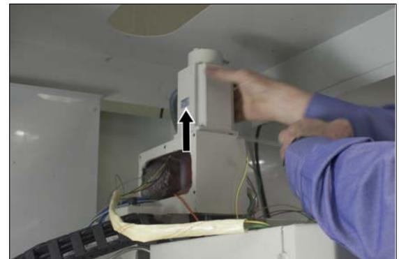
**Figure 1-14: Z-axis motor on the Z-axis motor mount.**
