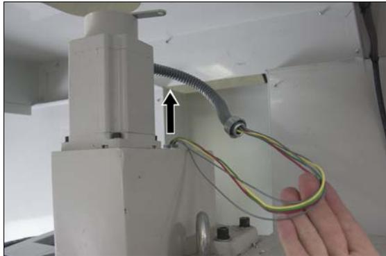
**Figure 1-11: Z-axis motor and brake wires inside of the Z-axis motor cable connector.**
