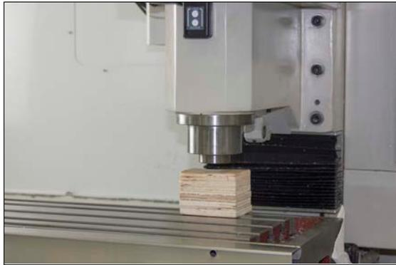
**Figure 1-2:** Example of a shipping block placed below the spindle nose.
