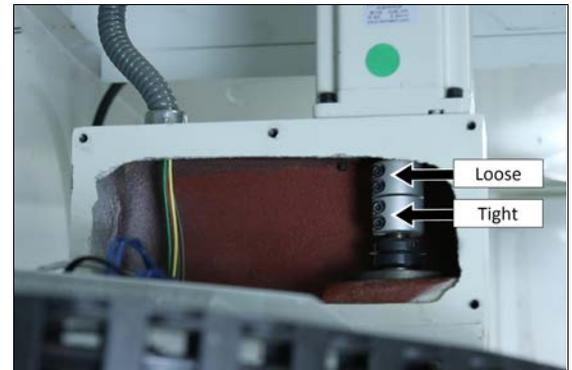
**Figure 1-13: Z-axis motor coupler set screws.**
