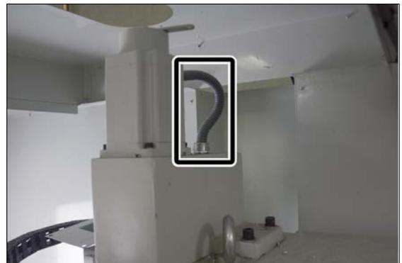
**Figure 1-10: Z-axis motor cable connector.**
