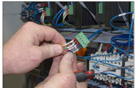
Figure 1-6: Z-axis motor wires on the Z-axis motor driver.
