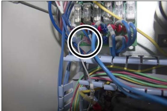
**Figure 1-7: Brake wire on the DC-BUS board.**
