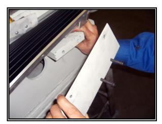
11. Hold the front end of the bellows tight to the joining plate. Scratch the positions of threading holes, then remove the supporting plate, drill and tap with the 3.3mm drill and M4 tap.
