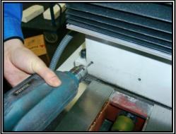
6. Use the screw driver to tighten the cover onto the column with the cross slot pan-headed screw  $M4\times12$ .
