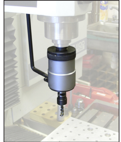
Fig. 1. Reversing Tapping Head
